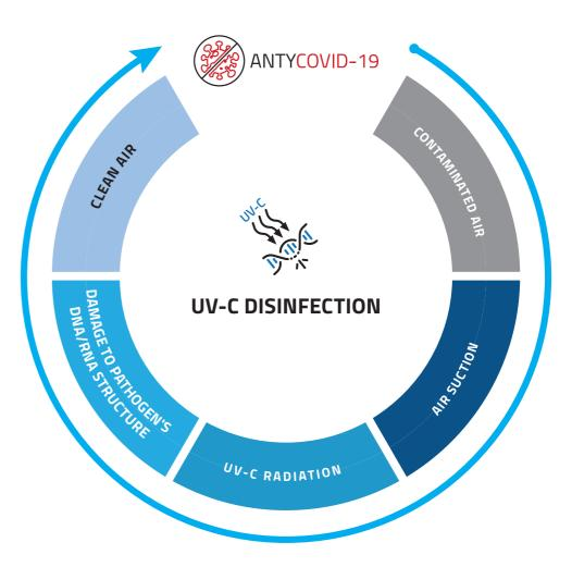
After passing through the disinfection duct of STERYLIS LIGHT AIR, the air is purified of any viruses, pathogens, fungi and moulds. STERYLIS LIGHT AIR luminaire has been optimised for a unit dose of > 50 J/m2 - scientifically proven to be effective in destroying the SARS-CoV-2 virus.
