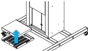
4. Remove the air filter from the cartridge
