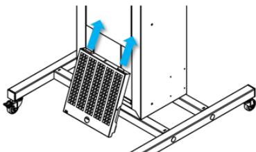
6. Turn the air filter cartridge as shown in the picture opposite and put it back into the device
