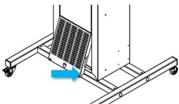
7. Push the cassette into the device housing
