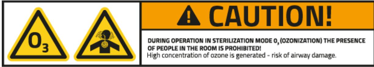
The device is designed to sterilise rooms by generating ozone in a concentration that may pose a threat to the health and life of humans and other living organisms. Despite the safety principles during the operation of the product as described in the following chapters, **it is essential to read the information below on possible effects of ozone and on first aid in case of exposure to a hazardous concentration of the substance.**
