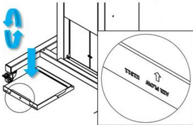
5. Insert a new air filter into the cartridge, making sure that the direction of the arrow on the cartridge and on the filter are aligned.
